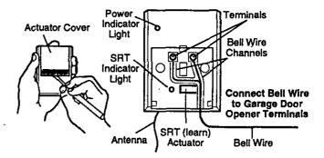
**OPEN RECEIVER:** Insert a small screwdriver in slot on receiver front panel as shown. Twist up actuator cover.
